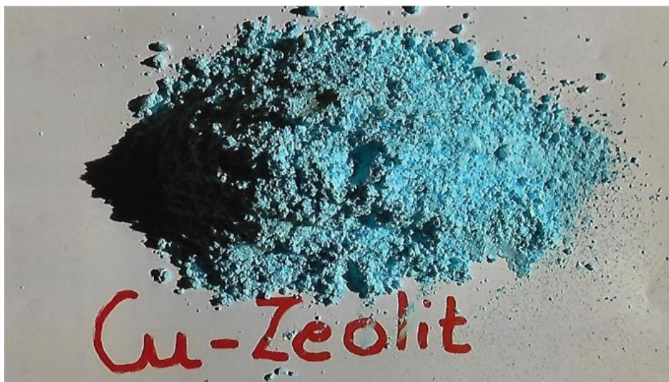
Figure 5.: Ion-exchanged zeolite with powdered copper-amine-complex ion, (self-photograph)
